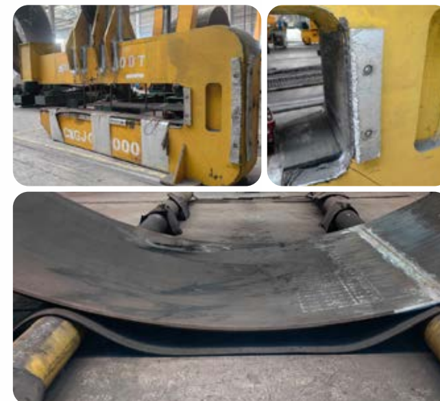
Hook with a Protective Layer and the Rubber Buffer Zone
