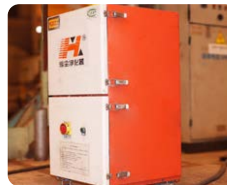
Mobile Welding Fume and Dust Collection Device
